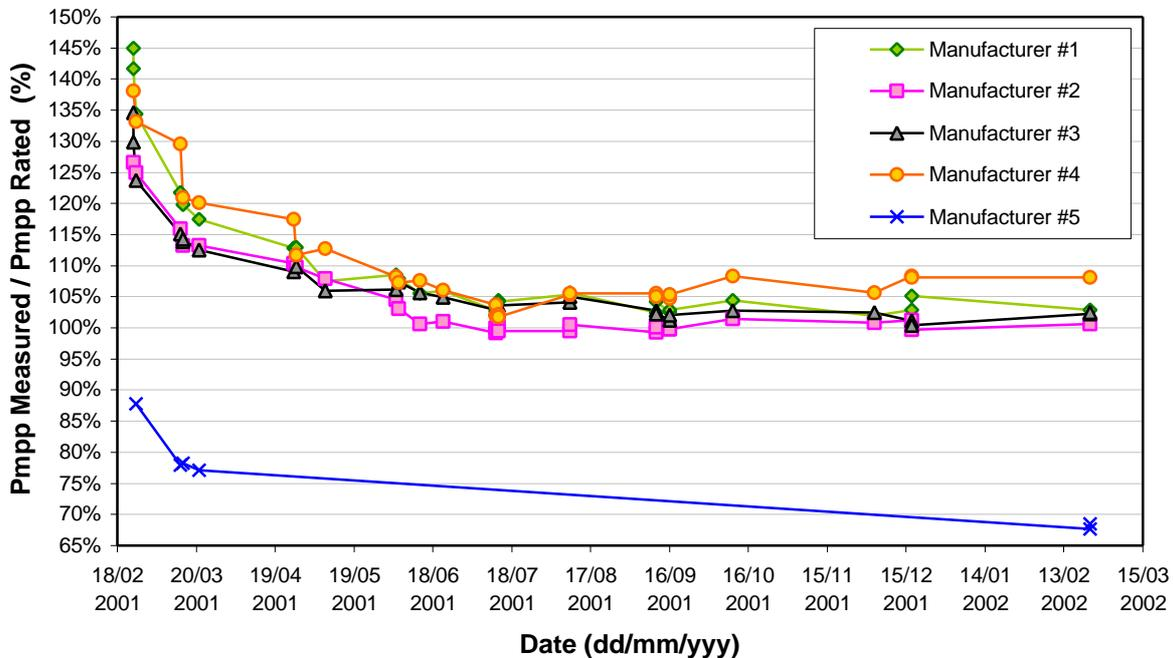
**Figure 5:** Evolution of the normalized output power (ratio of the real operating output at maximum power point measured outdoors, normalized to STC, and the nominal – nameplate rating - power at STC), for the five different multi-junction, commercially available a-Si PV module types used in this experiment. Measurements carried out at LABSOLAR under outdoor conditions, with irradiation levels above  $850 \text{ W/m}^2$ .
