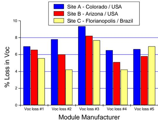
**Figure 2:** Losses in open circuit voltage (Voc) for the three sets of five different multi-junction a-Si PV modules after 12 months of outdoor exposure at the three different test sites. Measurements carried out at NREL under a SPIRE 240A solar simulator at STC.
