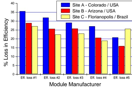
**Figure 1:** Losses in conversion efficiency for the three sets of five different multi-junction a-Si PV modules after 12 months of outdoor exposure at the three different test sites. Measurements carried out at NREL under a SPIRE 240A solar simulator at STC.
