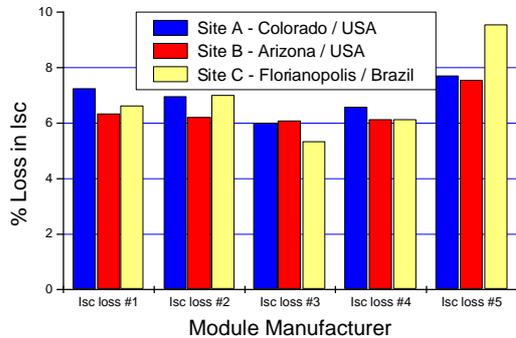
**Figure 3:** Losses in short circuit current (Isc) for the three sets of five different multi-junction a-Si PV modules after 12 months of outdoor exposure at the three different test sites. Measurements carried out at NREL under a SPIRE 240A solar simulator at STC.
