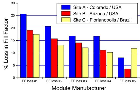
**Figure 4:** Losses in fill factor (FF) for the three sets of five different multi-junction a-Si PV modules after 12 months of outdoor exposure at the three different test sites. Measurements carried out at NREL under a SPIRE 240A solar simulator at STC.
